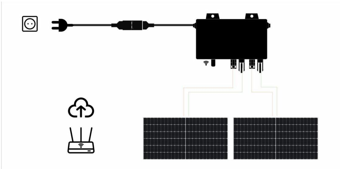
For balcony solution, there is only one inverter in the system. The monitoring is realized by WIFI connection between WiFi dongle on the inverter and home router.
